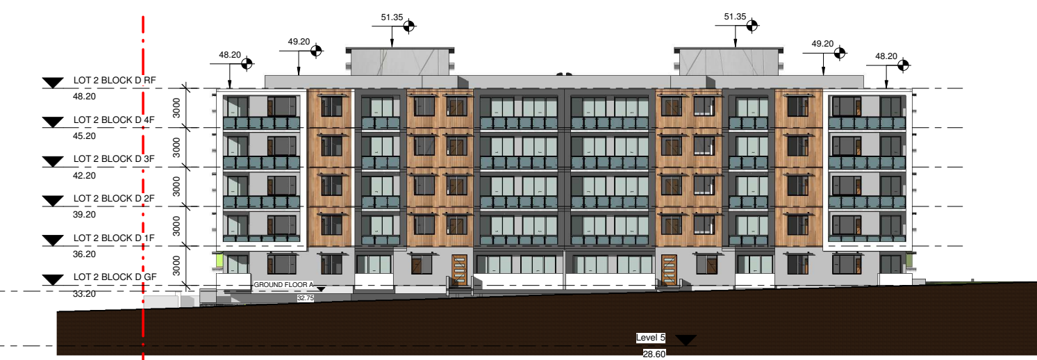
5 LOT2 BLOCK D EAST ELEVATION 1 : 200
